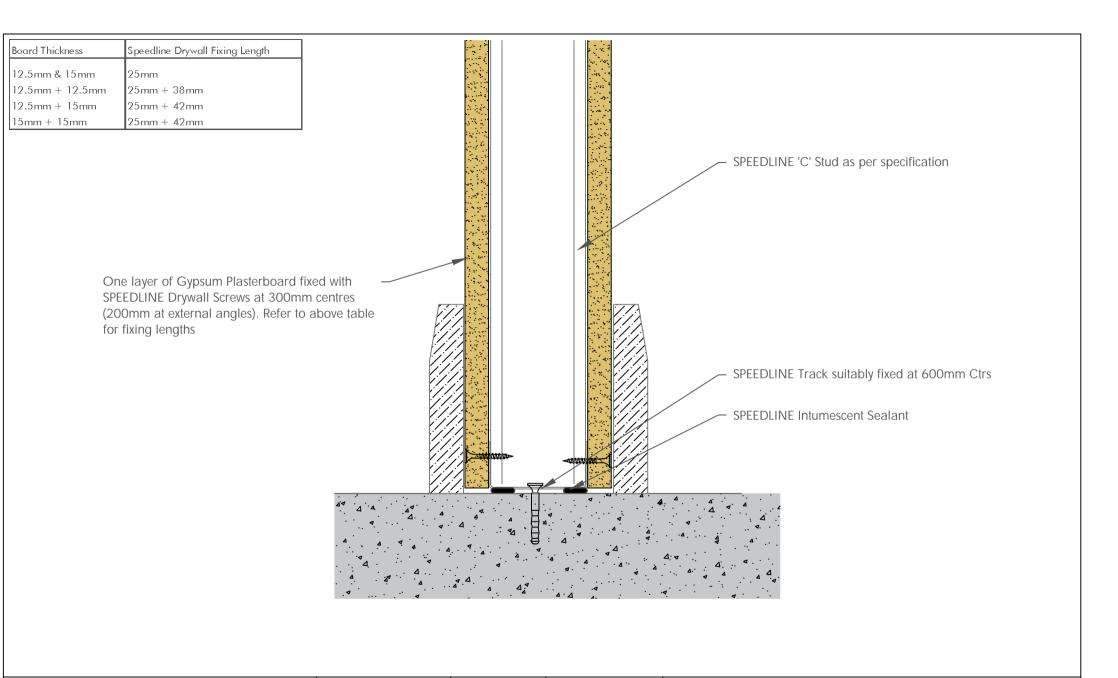
Detail may not replicate a laboratory tested configuration and for this reason approval from the relevant authority and Principal Designer should be sought
