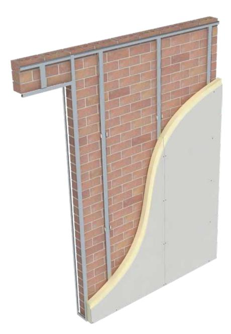
Speedline Thermal Laminate Board provides a thermal insulation solution in a single application and is suitable for use with Speedline Wall Liner System.
